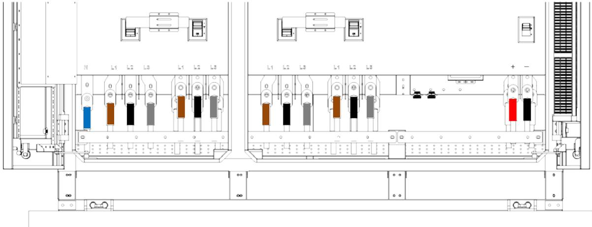
**Figure 4-11 Install the AC/DC cables**
