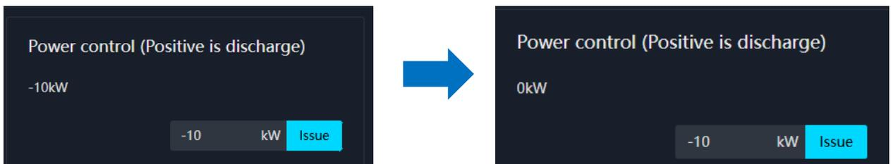
**Step 4:** Check the "Home" screen to verify that the PCS is in inactive mode, indicating that the equipment has been shut down.
